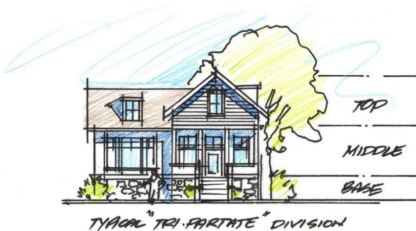
Figure 4: Definition: tripartite division in architecture is a design approach that separates a building's façade into three horizontal sections: the base, the middle, and the top.
