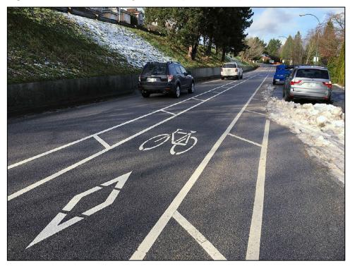
Figure 2.4 – Protected bicycle lane with parking (Vancouver)
