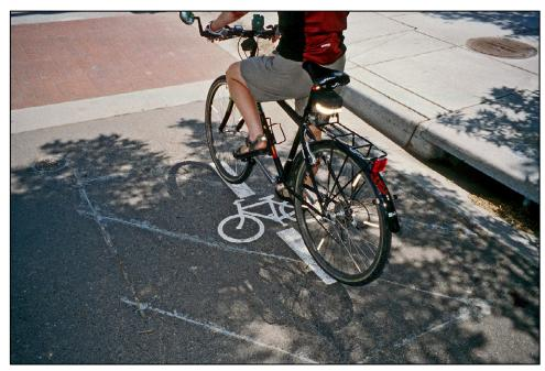
Figure 5.13 – Bicycle detector sign (Vancouver)
