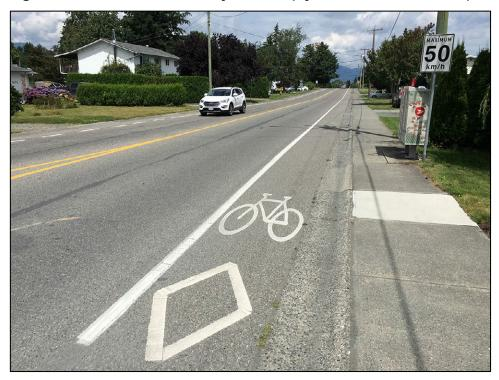
Figure 2.3 – Buffered bicycle lane (Vancouver)
