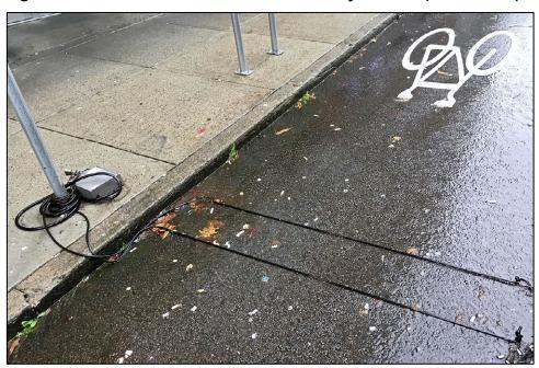
Figure 3.18 – Automatic counter across bicycle lane (Vancouver)
