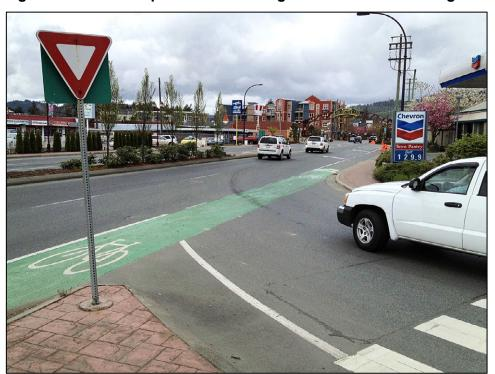
Figure 5.21 – Green pavement marking across channelized right turn lane (Langford)
