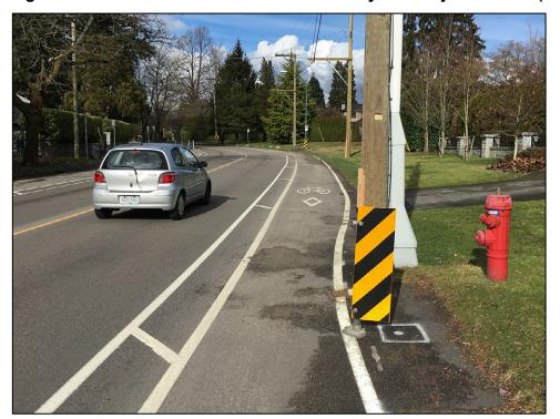
Figure 5.8 – Reduced width shoulder bikeway with object marker (Vancouver)
