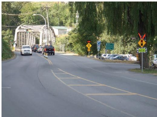
In response to a WorkSafe BC order a new traffic signal was installed on Vedder Road at Chilliwack Lake Road with a remote control feature to allow a flagger to manually control the intersection during peak traffic flow.
