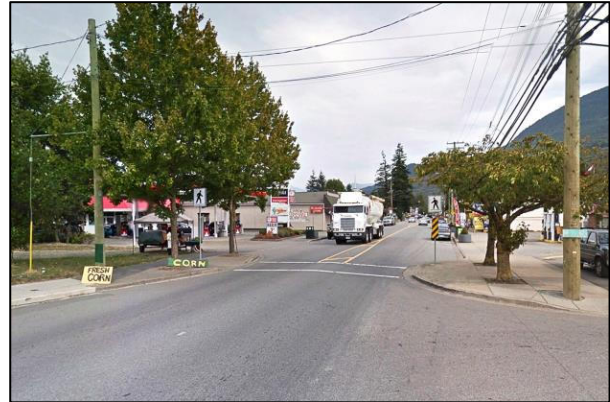
Figure M.2 Curb Extensions (Yarrow)
