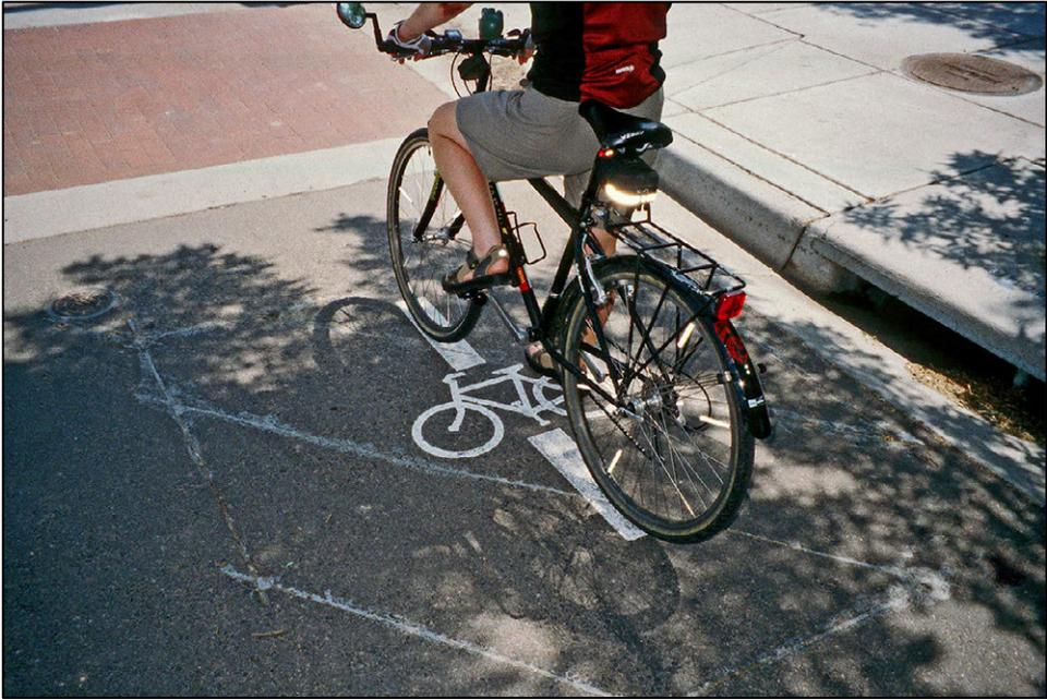
**Figure 5.13 – Bicycle detector sign (Vancouver)**
