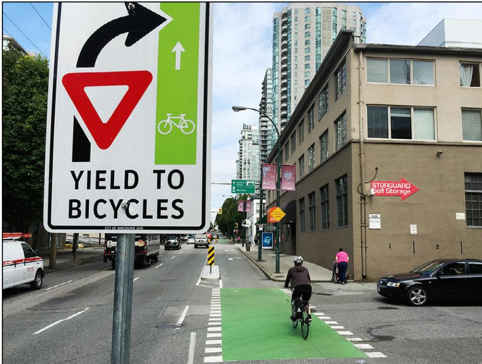
Figure 5.20 – Green pavement marking through intersection (Seattle WA)
