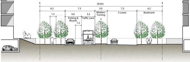
Figure 3.18: Cross section option for a 30m right of way
