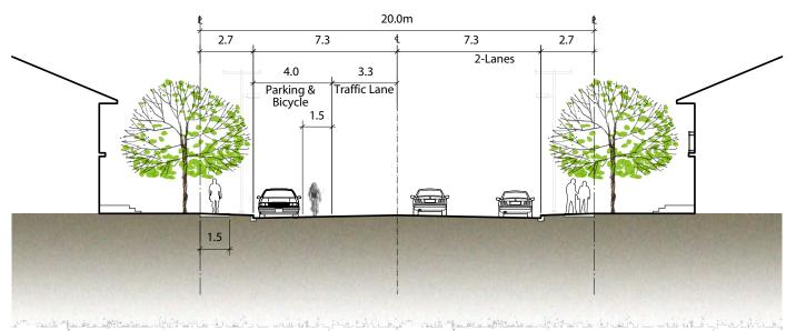
Figure 3.14: Green link corridor cross section - 2 travel lanes, bike lanes and parking with wide sidewalks for easy pedestrian travel. Street trees provide shelter and 'green'.
