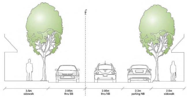
Figure 3.13: Preliminary design for Mill Street Mews (above) and illustration of zones (below)
