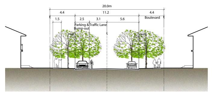
**Figure 3.16: Priority for Bicycles and Pedestrians**. Options could include a 'bump out' in a greenspace, take over a parking stall or extend corner bulges for pedestrians or install center greens on streets where traffic volumes are low, where traffic speeds should be calmed - i.e. near parks, seniors centres, hospitals, etc., and where street parking is less used (as in single family neighbourhoods).
