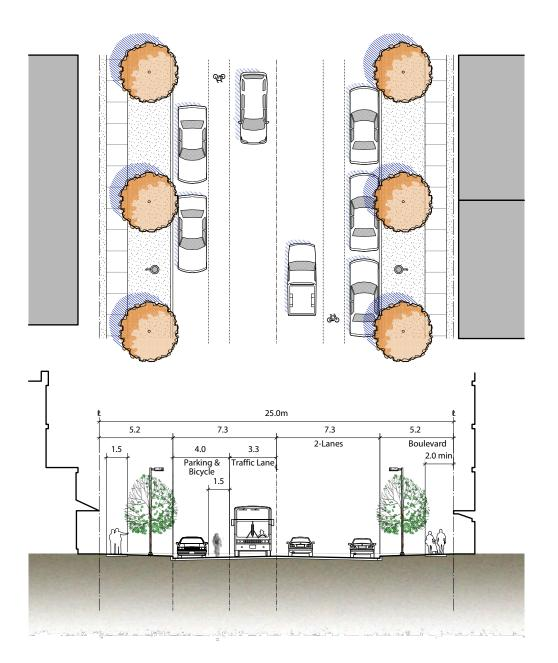
Figure 3.4: Major Arterial Conditions - 25m right-of-way
