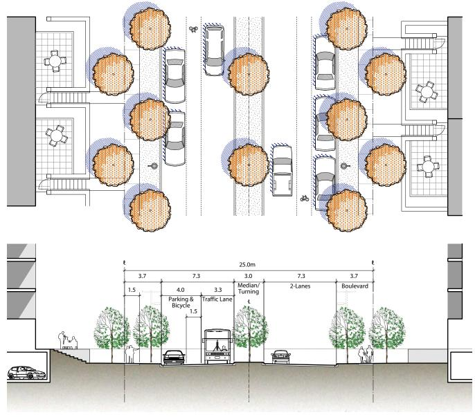
**Figure 3.19: Spadina Boulevard Extension** - option for a 25m right-of-way (20 m in between Mary Street and 1st Avenue. Street trees are located within both public and private realms.
